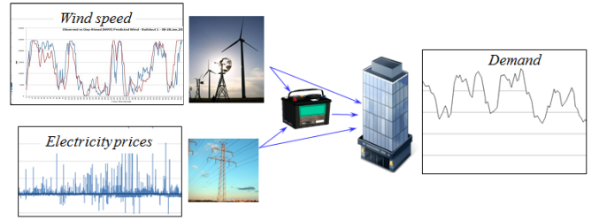
Fig. 1. Storage system with energy from renewables and the grid to serve a time-varying load, with a storage device.
